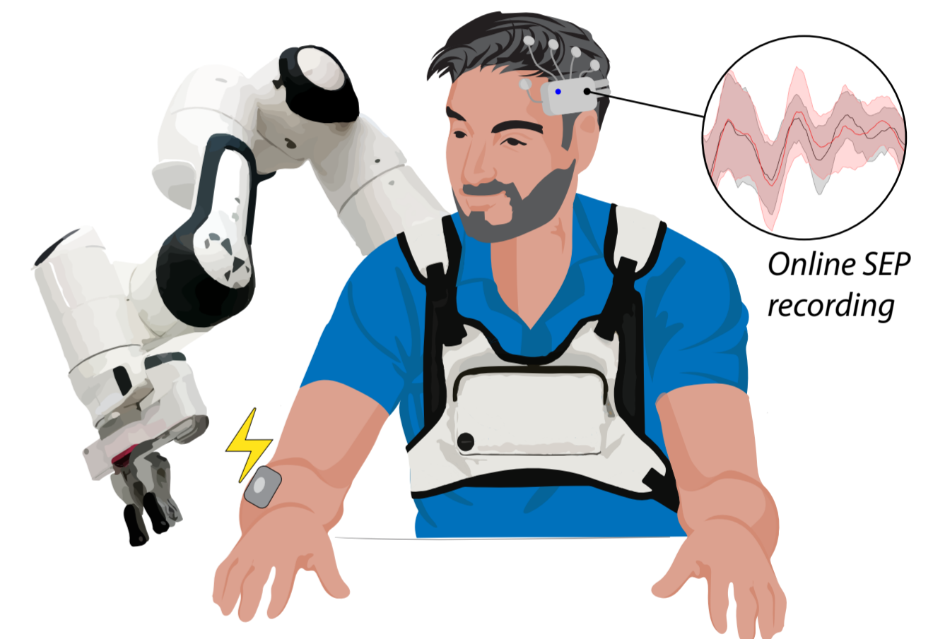
Figure 3. Conceptual setup for testing embodiment of SRL through SEP attenuation. The somatosensory feedback encoding the SRL status is exploited to elicit a measurable SEP that can provide an online marker for embodiment.
