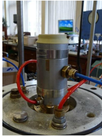
Membrane rolled around mould and suction applied
