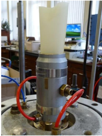
Mould placed around membrane
