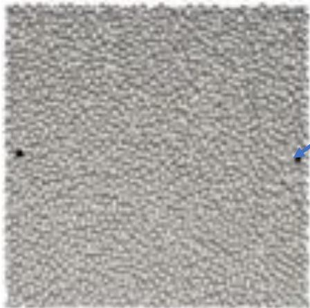
Bender element modelled as point source (particle)
