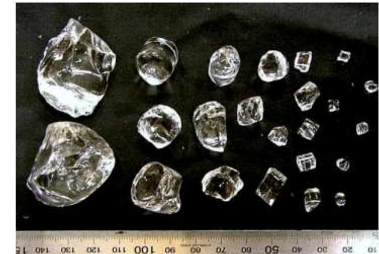
Model soil – crushed borosilicate
