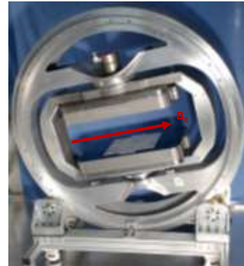
Figure 1: A photograph of the prototype scanner - an open MRI system with the main field B_0 parallel to the poles (red arrow). Two motors rotate the magnet about two orthogonal axes allowing B_0 to move around the patient.
